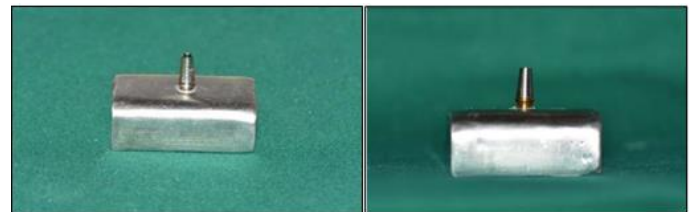
Figure 3: metal model with implant and abutment (Adin parallel connection and osstem conical connection)
