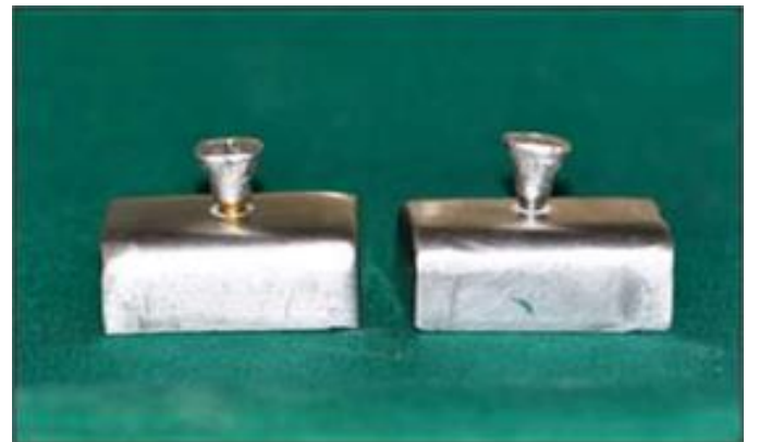
Figure 4: a) metal mounting jig fabricated on abutments b) cyclic loading
