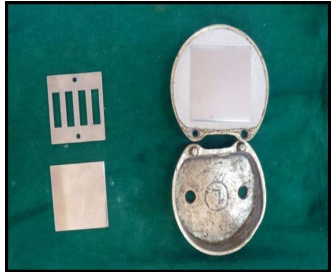
Fig. 11: Flasking with Metal Mould
