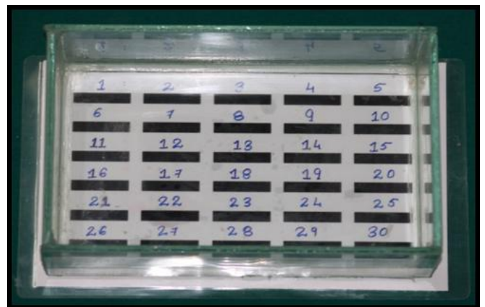
Fig. 18: Custom made samples guide placed beneath the beaker
