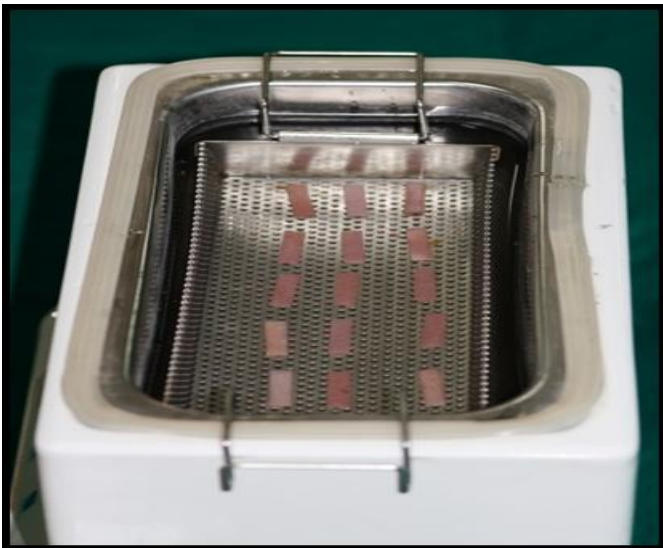
Fig. 21: Samples Placed in Ultrasonic Denture Cleanser
