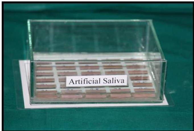
Fig. 19: Samples Placed in Artificial Saliva
