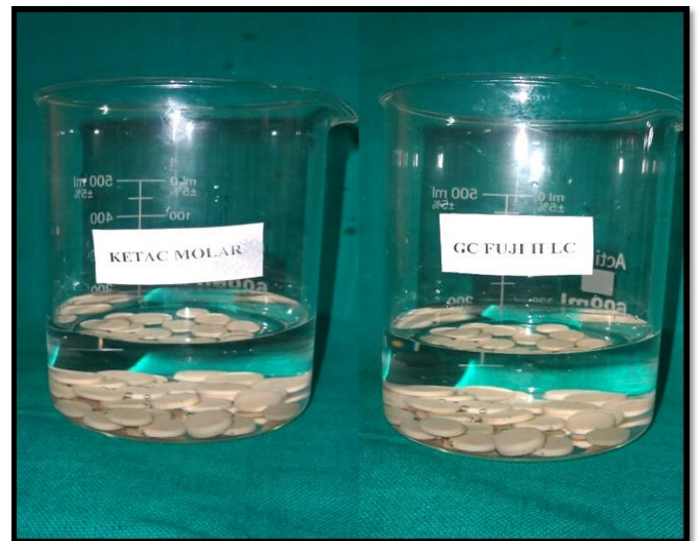
Figure 5: Rehydration of samples by placing them in distilled water for 24 hours.
