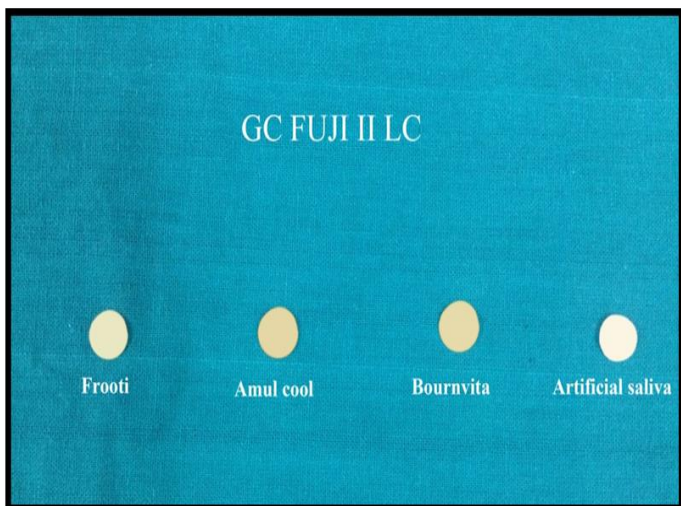
Figure 10: Showing color difference seen at the end of day-15 in specimen of GC FUJI II LC.
