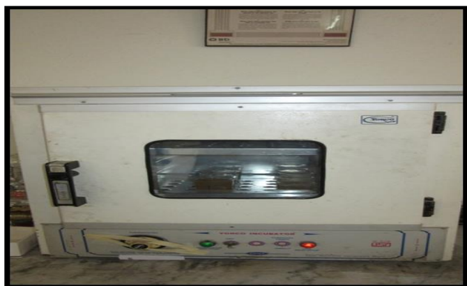
Figure 7: Specimens kept inside incubator at 37°C temperature.
