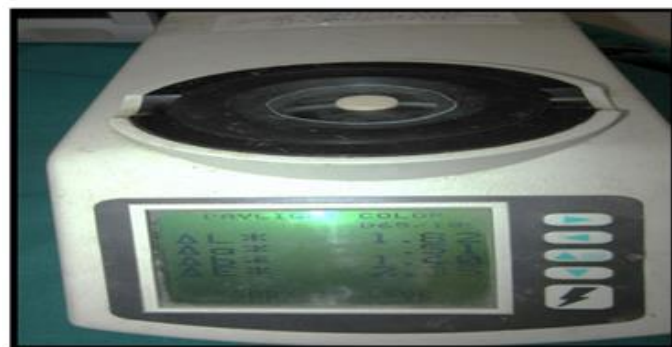
Figure 8: Color difference \Delta E calculated using spectrophotometer.
